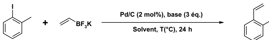
Scheme 2. Heterogeneous Pd-catalysed vinylation of o -iodotoluene.
